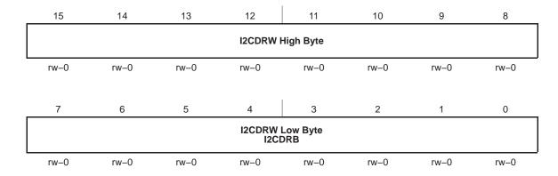
I2CDRW/ I2CDRB Bits 15–8  $I^2C$  Data. When I2CWORD = 1, the register name is I2CDRW. When I2CWORD = 0, the name is I2CDRB. When I2CWORD = 1, any attempt to modify the register with a byte instruction will fail and the register will not be updated.
